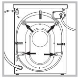
Remove the 4 protective screws (used during transportation) and the corresponding spacer, located on the rear part of the appliance (see figure).
